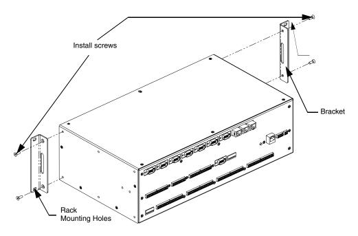
FIG. 22 Mounting Integrated Controller into an equipment rack
